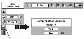
Move the pointer to Lamp counter reset and then press SELECT button. The message "Lamp replace counter reset?" is displayed.
